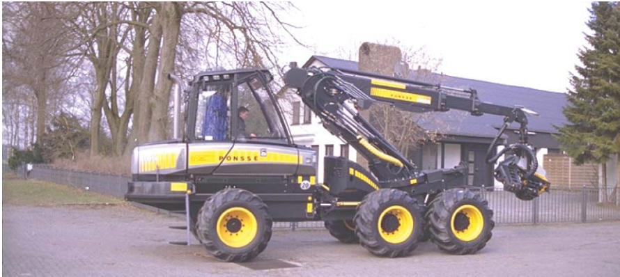
Figure 4. Ponsse Beaver harvester with different operating and driving directions.
