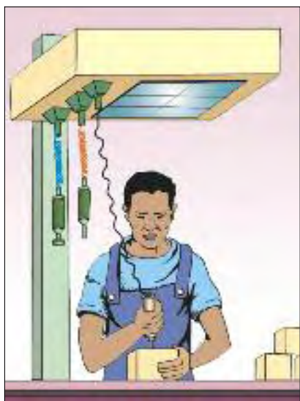
Figure 20c. Provide a special overhead frame from which tools can be hung by means of spring mechanisms.
