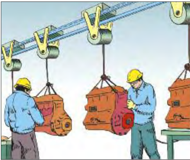
Figure 10a. Mechanical transport of materials can both eliminate manual work and improve work height and working posture.
