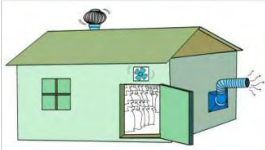
Figure 93a. Supply sufficient airflow to confined work areas where oxygen deficiencies may occur before entering there.
