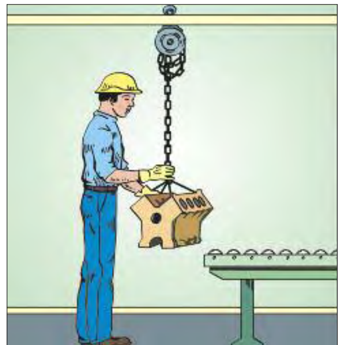
Figure 9d. Make sure that the maximum safe working load is plainly marked.
