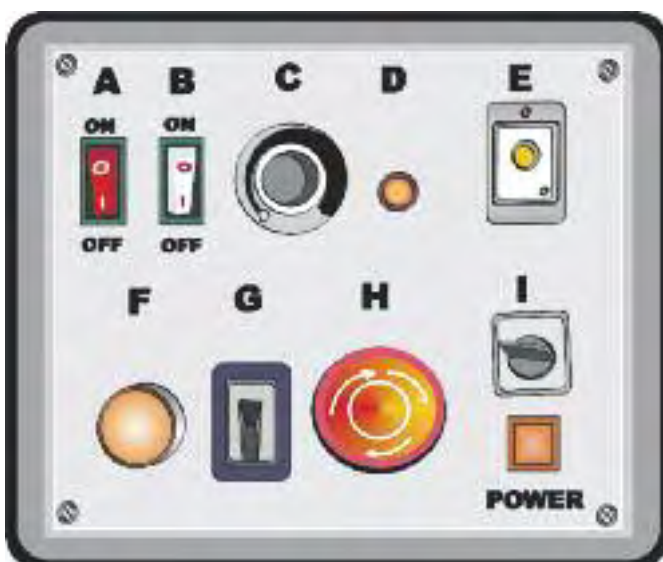
Figure 34b. Examples of making different controls easier to distinguish from each other by changing their shapes and colours.
