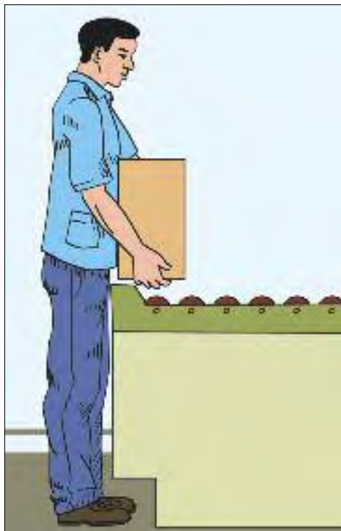
Figure 5b. Rollers or conveyers can reduce the distance materials have to be moved manually. The height should be such that the work item can be handled without bending the upper body. Make sure there is enough space for the feet and body to get close to the rollers or conveyers.
